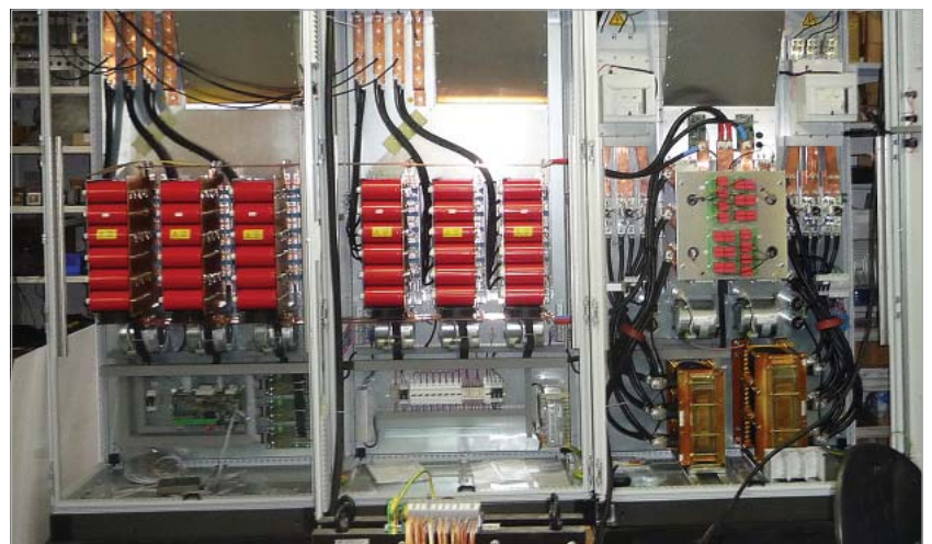
Custom built frequency converter UNIFREM 720 1400 for special motor (720 V, 680 A, 1400 kW, 11000 rpm, 184 Hz)
